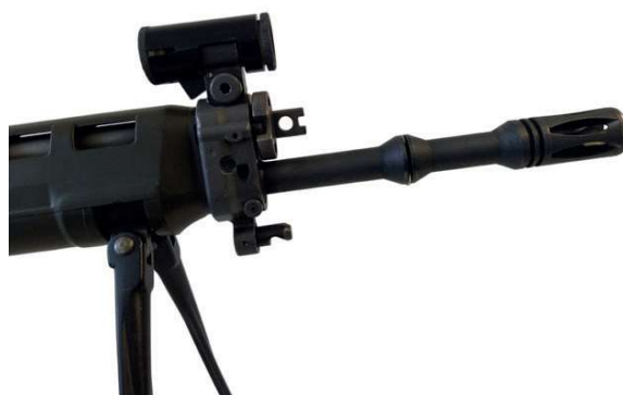
Figure 9: Guidon annulaire Zumkeller
